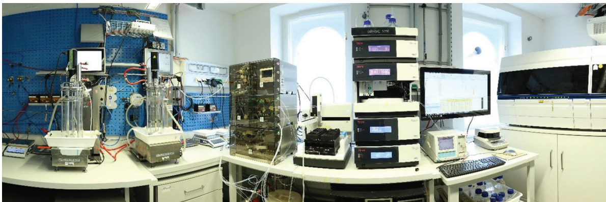
Figure 2-2: Set-up example for a PAT-bioreactor system with extensive on-line analytics, fully automated by Lucillus PIMS. The set-up includes a Numera system that is connected to an HPLC and a biochemical analyzer to facilitate automated sampling as well as on-line measurements of substrate, metabolites, products etc.
