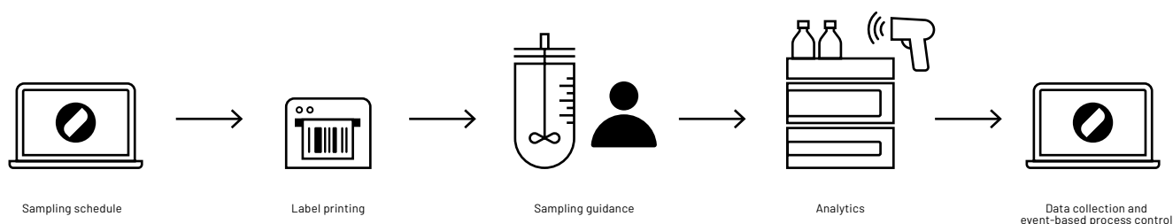
Figure 2: Sample management workflow with Lucullus®. In Lucullus® a sampling plan is defined and a unique barcode for each sample is generated. The barcode is printed as a label and the respective sampling tube is labeled. The operator is then informed by Lucullus® to take a sample at a predefined process time or process event (sample guidance). The barcode of the sample is
