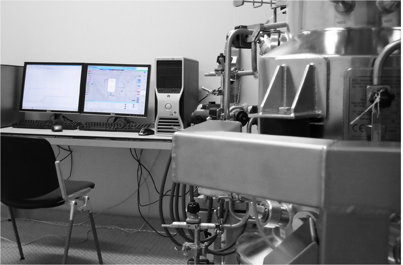
Illustration 3: Plant control and process monitoring in production with Siemens WinCC and Lucullus®.
